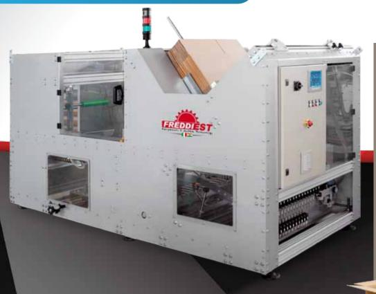
FC/12 Case Erector is designed to erect CFC corrugated carton with different sizes. Attraction in the machine is its user friendly Technology, Reliability, Repeatability and fast change in different carton sizes from Smaller to Big carton. Unique adoptability of Freddi machine is "Machine can integrated with Pick & Place attachment as it will be called as Monoblock Case Packer".
